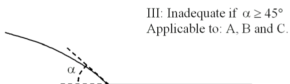
Figure C-7 Weld metal cap profile
